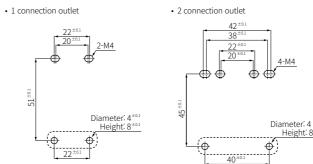
is installing spot of protrusion for fixing the switch firmly.
